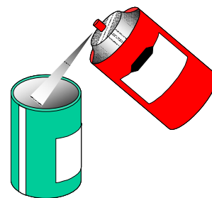
図-1 型枠内面へ潤滑剤を噴霧
